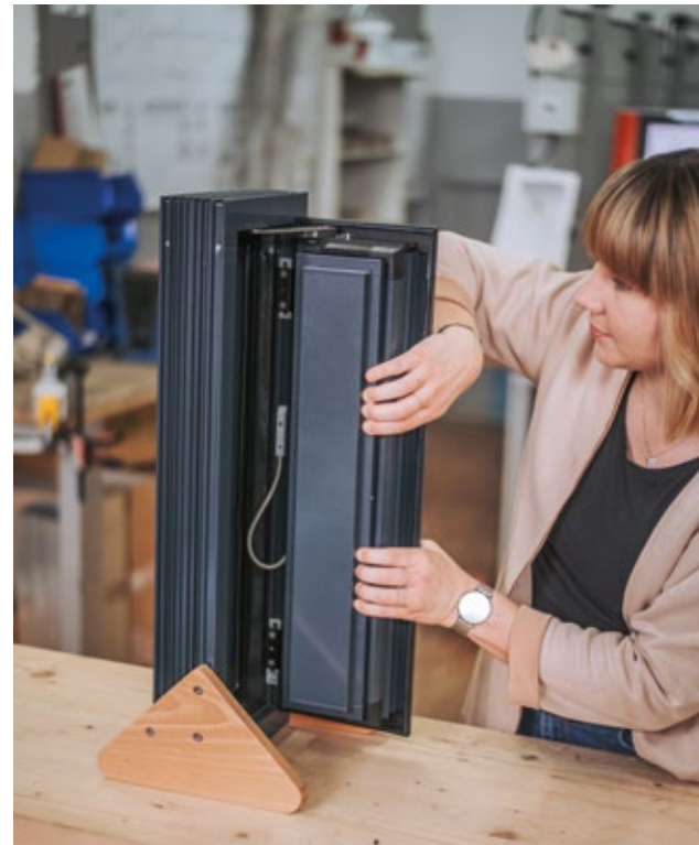
THANKS TO THE DECOUPLED INTERIOR AND EXTERIOR SHELL, THE BI-METAL EFFECT IS REDUCED TO A MINIMUM
